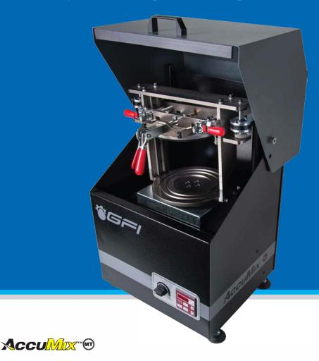
The AccuMix-MT makes quick work of thoroughly blending formula components together to provide a tool-free means of mixing materials together. After your AccuBlend-HV doses the formula into a standard 5 or 10 pound (2.5 kg or 4.54 kg) metal tin, it is clamped into the AccuMix-MT. From there, about five minutes is all it takes to get ink that's ready to take to press.
